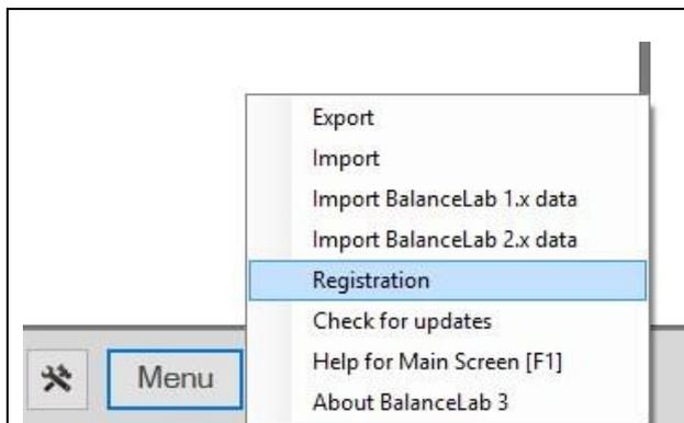
1. Check if the right BalanceLab hardware (pressure plate) is connected to your Laptop/PC: Choose "Registration" in the "Menu" section of the main menu.
