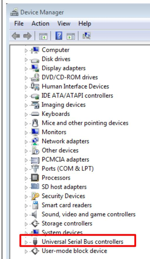
3. In the list of devices go to the bottom to "USB-Controller" or "Universal Serial Bus controllers". Expand the field (+) if necessary.
