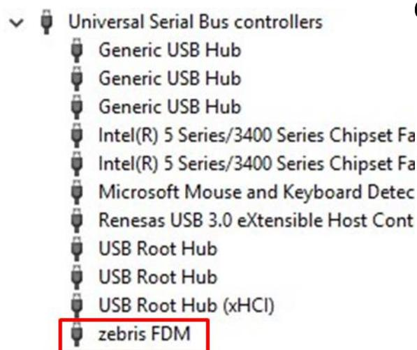
6. After the driver installation is finished the entry in the device list should change to what is shown in the left picture.
