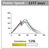
Average putter speed exactly at Impact. The curves show the course of putter speed in the forward swing. The vertical stripes represent impact.
