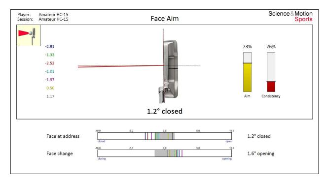
The graph shows the alignment of the **putter face at address**. The dotted line exactly represents the calibrated target direction. At 0 degrees the putter face is 100% square to the target. The average direction of the putter face alignment is represented by the thick red line. The area between the average alignment and the optimum target direction is filled in red color to indicate the amount of deviation.
