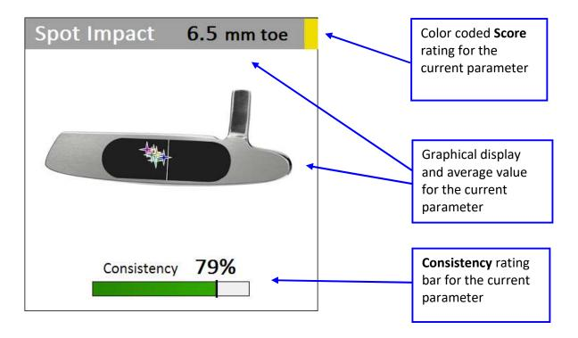
If using S-Tiles during training the consistency bar is blinded out, and instead the actual data value is displayed in the center of the tile:
