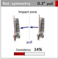
Average rotation symmetry in the impact zone, which is the difference of rotation before impact to rotation after impact. The pictogram represents the symmetry in 5 grades with additional description (here "pull").
