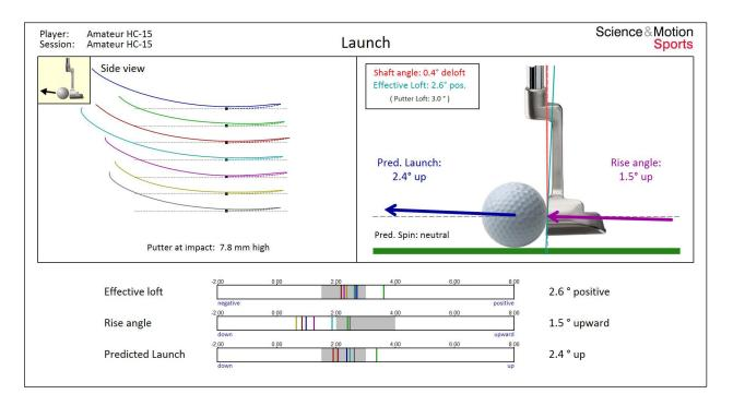
The left graph shows a **horizontal side view** of the putter path during back swing (dotted lines) and forward swing (solid lines). The different putts are indicated by different colors, with the first putt at the top. The physical horizontal ground is indicated by horizontal grey dashed lines.
