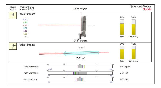
The Direction report summarizes the data from the Face at Impact and Path at Impact reports. Face angle and path direction can compensate for each other. A path which is not pointing exactly to the target can be compensated with a face pointing into the opposite direction to make the ball still go straight. For this player in fact the face is pointing to the right which is compensated by the path pointing to the left.
