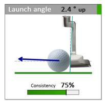
Average calculated Launch angle at Impact based on effective Loft and Rise angle at Impact. The graph and the arrow represent the true angles.
