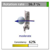
Average rate of rotation (rotation speed) exactly at Impact. The pictogram represents the amount of rotation in 5 grades with additional description (here "moderate").
