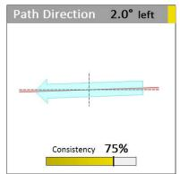
Average putter path direction angle exactly at impact. The arrow represents the deviation from the optimum.
