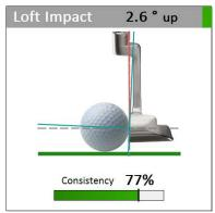
Average effective Loft at Impact. The graph represents the true angles. The effective loft is the sum of the static Loft and Shaft lean.
