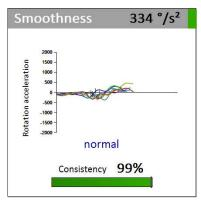
The smoothness of face rotation is described by the amount of rotational acceleration around impact. The data curves show the course of rotational acceleration in the forward swing. Severe irregular oscillations around impact can indicate Yips problems.
