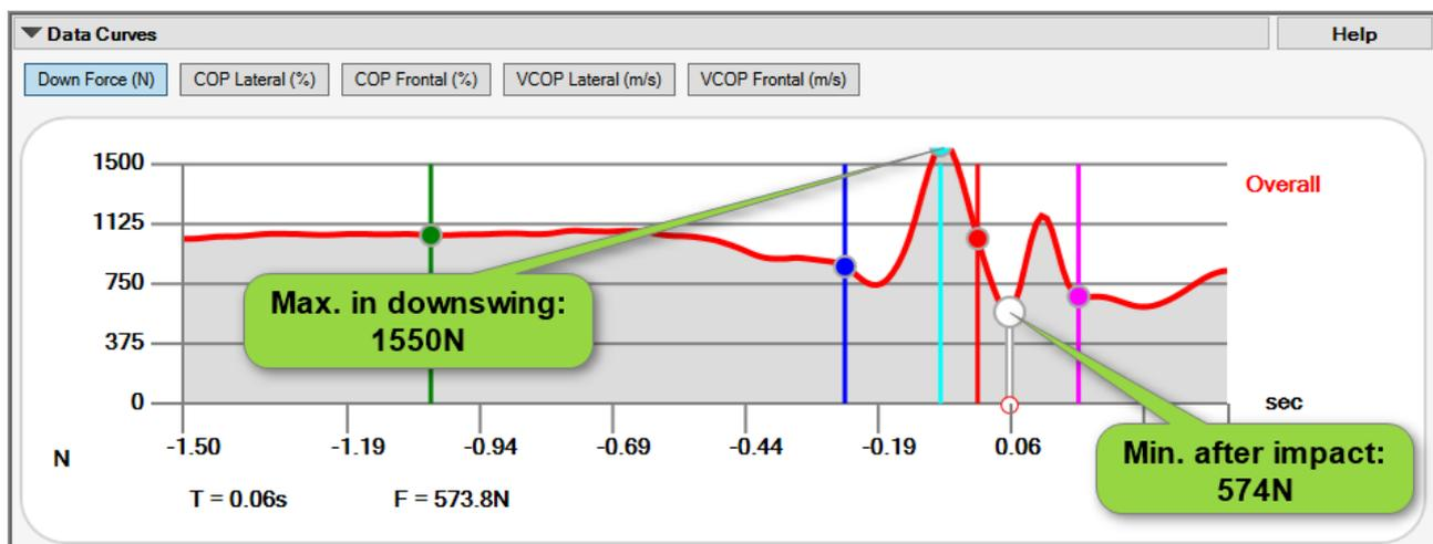
The scale at the left is indicating the overall downforce in Newton. The horizontal scale is representing the time in seconds relative to impact. Impact is exactly at a time = 0 seconds. The data under the graphs show the time and the down force at the actual cursor position.
