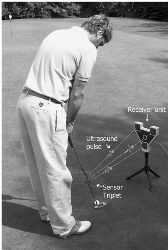
Figure 1. Measurement Principle of SAM PuttLab
